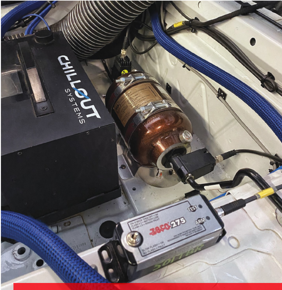
Shown here is an example of an electrically activated FIA system typically seen in sports cars and road racing. System installation should follow both the sanctioning body's rulebook as well as the system's instruction manual to achieve the intended performance.
