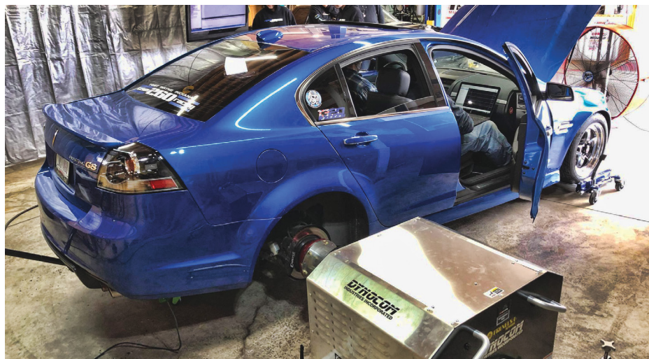
Dynamometers can be a big revenue source for shops of all sizes. Setups like this Dynocom portable unit are well suited for tight spaces and temporary locations.
