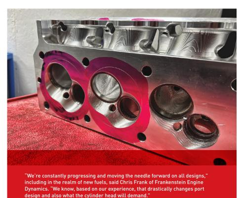
Our head is currently .500-inch thick. With the increase in boost levels and horsepower, we've raised the deck thickness to .750-inch. We also made revisions to the water jackets to allow a larger port."
