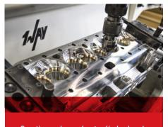
Creating a clean-sheet cylinder head can require months of development work. 1 Way Technologies discovered new efficiencies when it came up with a way to produce GM SB2 and ROX cylinder heads from a single casting.
