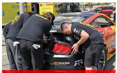
Because contact is not uncommon in drifting, most teams bring spare aftermarket bumper structures and other body components to make them easier to replace between heats, "especially for the rear," said Kevin Wells of Formula Drift.
