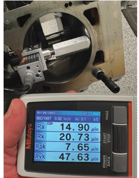
The human eye can't see objects smaller than .002 of an inch, so a profilometer, which measures roughness down to a millionth of an inch, is needed to accurately measure surface finish. (A fingernail isn't accurate enough.)
