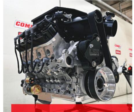
The LS engine block offered by RHS was built to withstand extreme boost by utilizing premium aluminum in its construction and six-bolt steel main caps, which are designed for increased clamping strength.
