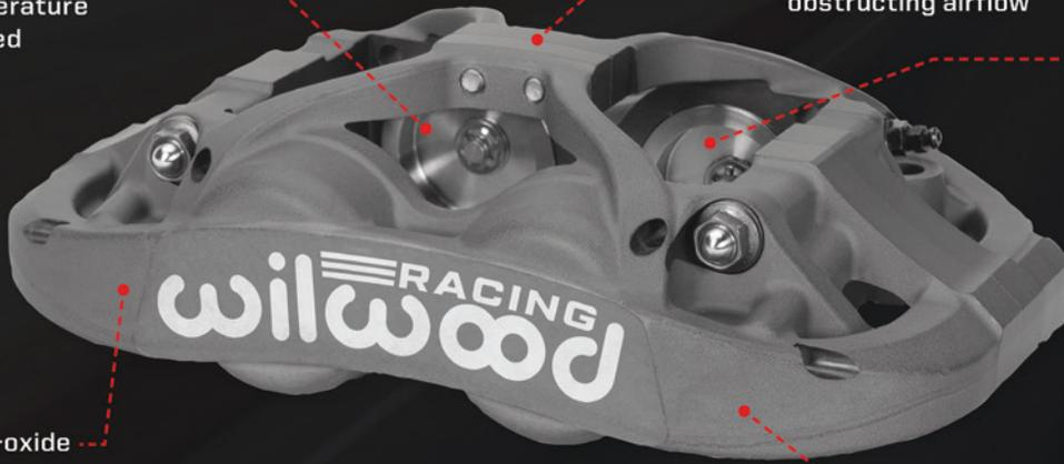
Durable aluminum-oxide ceramic Type III hard-anodized finish
