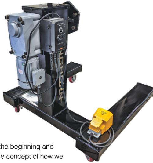
"We started from the beginning and redesigned the whole concept of how we rotate engines," said Manfred Schreyer, "much of which is side mounted to allow an engine to be bolted to the stand by only taking off one motor mount."
