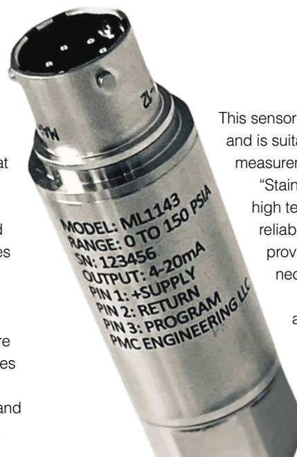
This sensor also uses piezoresistive silicon technology and is suitable for static and dynamic pressure measurements with a frequency response of 1ms.
