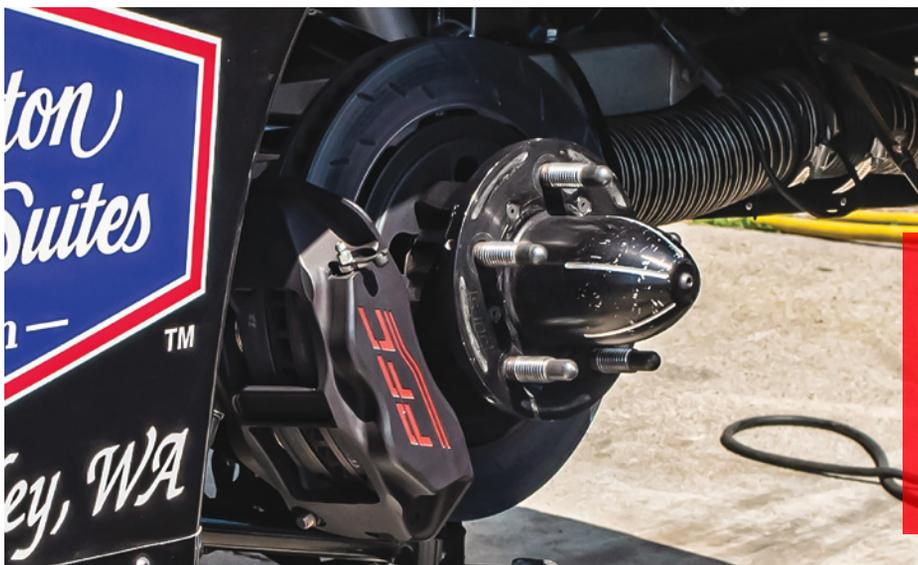
The monobloc brake calipers made by PFC Brakes for short track use are stiffer and more rigid than a two-piece caliper, said our source, which means they require less maintenance over time. The calipers also improve brake feel, since only the pistons are moving, not the caliper parts.
