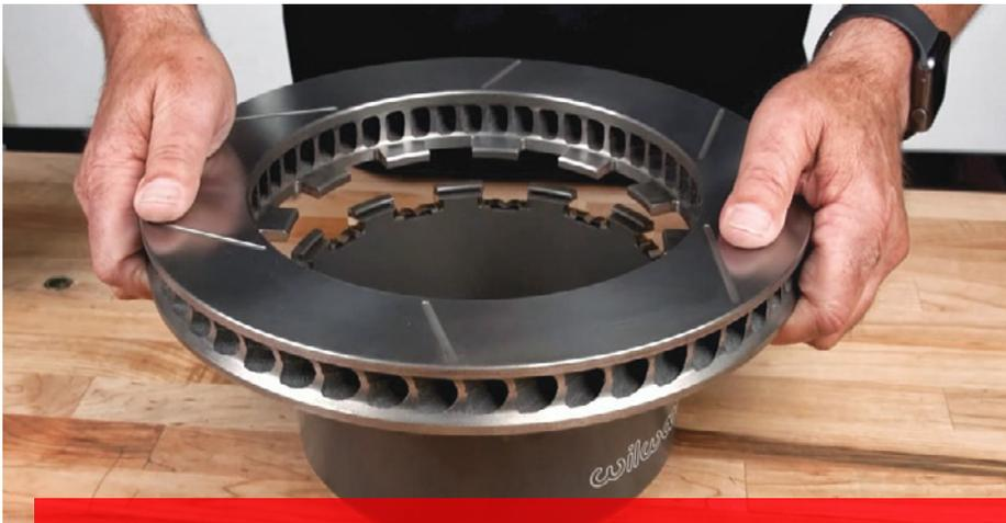
Wilwood's new Lug-Drive Dynamic Mounting System replaces the traditional hardware used to mount a rotor to a hat with a single internal snap-ring. With the new system, rotor changes can be done quickly and with no tools, said our source, and the service life of the hat and rotor are extended thanks to a reduction in the distortion that can be caused by thermal cycling.
