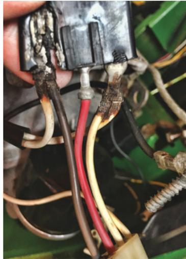
which causes numerous problems." A better approach, he said, is "grounding to the battery directly if possible, or having a welded stud on the chassis frame or whatever they might be working with. When it's welded and properly cleaned and prepared, it's a more durable ground that will have a better connection."
