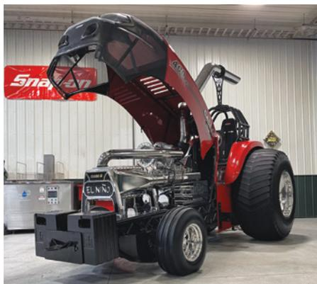
The engine in Colin Ross' "El Niño" Pro Stock tractor is based on an International DT466 inline six, but it was designed at Chaos Fabrication and cast for Ross. "We saw a lot of areas in the blocks we were using that needed improvement, so we took it upon ourselves to create our own." Dyno testing is essential for these pulling teams, Ross said. "Horsepower doesn't guarantee wins, but it sure doesn't hurt to have all that you can get."
