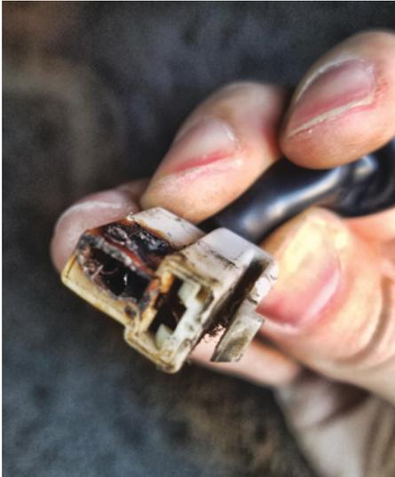
According to our source at SPAL Automotive USA, when working with connectors it's important to "avoid dielectric grease or anything like that inside the connection because of the fan's heavy current load." This, he told us, can cause corrosion or arcing at the terminals, among other problems; it can also "cause the grease to wick up and down the wires."
