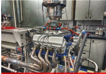
Analysis of the oil in Lake Speed's NASCAR Ford showed water in the oil, which came from a tiny crack in one of the intake runners. The engine is now back from the dead and making more power than ever.
