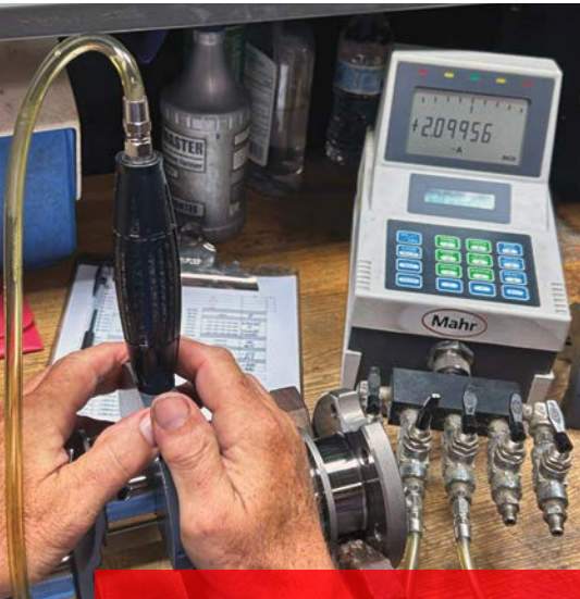
Part of the final crankshaft inspection at Manley Performance Products includes an air gauge to double-check journal sizing.
