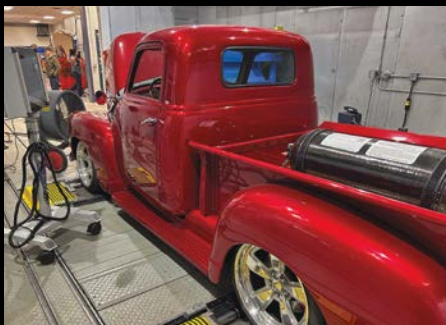
Mike Copeland fuels the Magnusson-supercharged LS in his custom Chevy pickup with hydrogen. Its output is around 500 hp, and it has passed a battery of emissions tests. It actually emits less carbon than the atmosphere that surrounds it.
