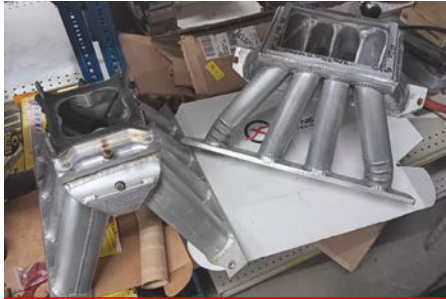
Weinle Motorsports continues to experiment with runner length and size when building intakes for dirt late models.
